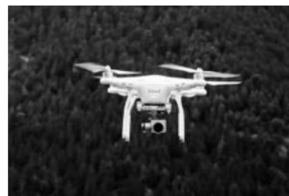
for this level of analysis cost is under \$2,000. Another option is attaching a more expensive (\$5-10K) multispectral sensor, which could allow the landowner to visualize the "stress responses" of individual trees. This gives researchers the ability to make inferences about drought, disease, and nutrient deficiencies. In a broad sense, this will likely become a vital early detection tool for foresters.
